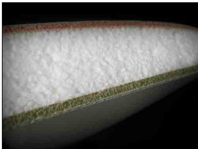
Full sandwich construction for maximum weight loss and hull stiffness
